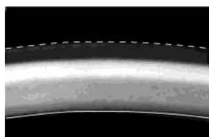
Figure 6. Asymptotic stable mixed state of the gel in the spatial bistability domain in the presence of malonic acid. Experimental conditions: [MA]_0 = 2 \times 10^{-3} , [I^-]_0 = 0.92 \times 10^{-3} .
